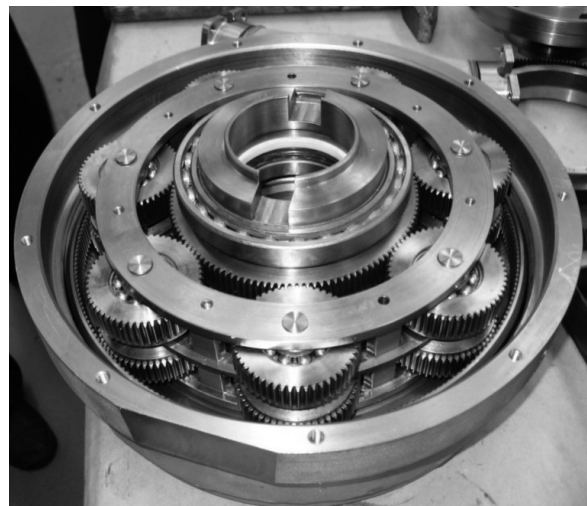
Fig. 1. A two-step planetary reducer of small module with 12 streams of type « 3k - 2g - h » with an open cover of a reducer of the multitaround electric drive of the third dimension with a connecting flange type B (□ 200×200 mm)
