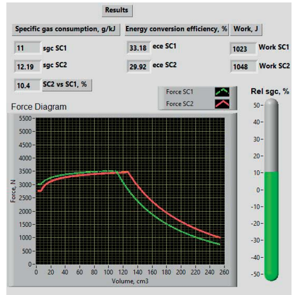
Figure 4. User interface of the model. Force – volume diagram and calculated efficiency parameters are shown
